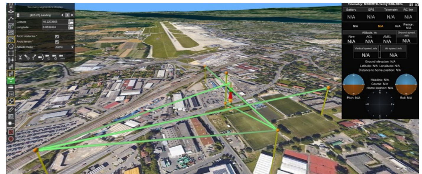
Vertical, Mini-Orbit and Mini-Approach trajectories for default maintenance procedure
