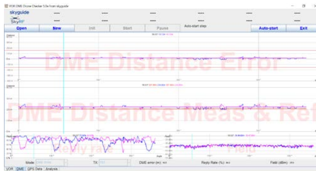
Figure 16: The VOR DME Drone Checker in the orbit mode (DME window)
