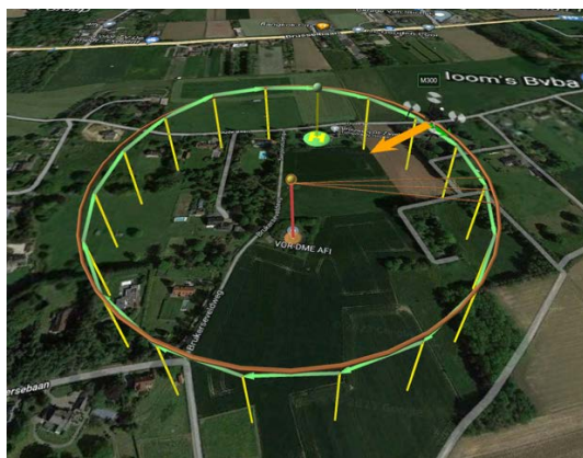
Figure 2. Illustrations of preconfigured waypoints in a general mission planning software
