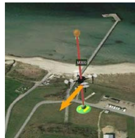
Figure 21: Vertical PAPI Flight Pattern
