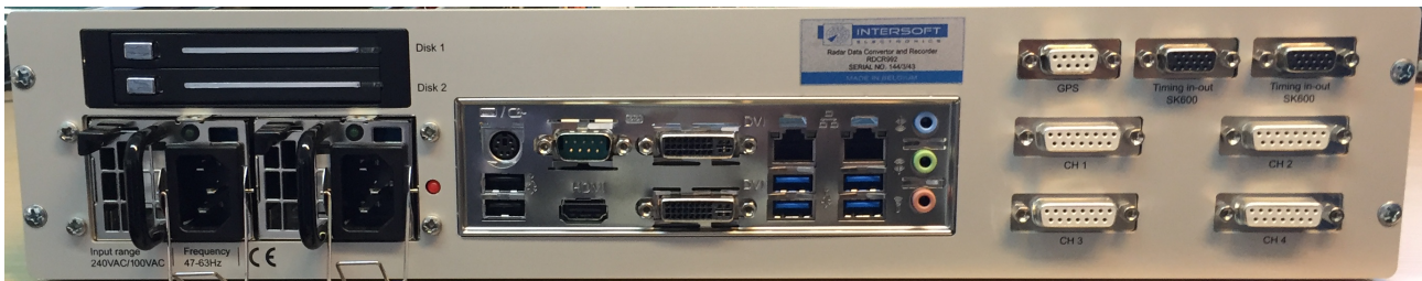
Figure 2.2: RDCR992 rear panel
