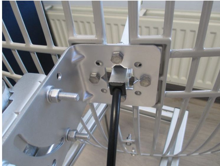
Figure 12: Step 3 – Install the L-bracket
