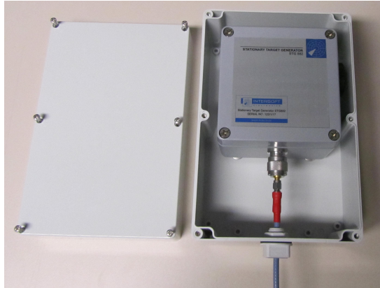
Figure 16: Step 3 – Installing the STG inside the plastic cover
