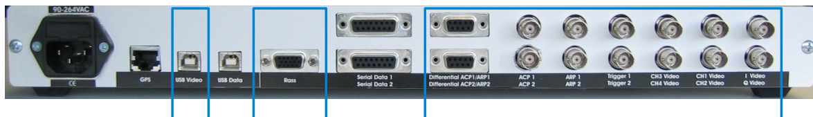
Figure 2: Rear panel RIM782 – Video Board connectors
