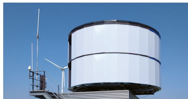
Figure 2 | Prototype of Intersoft Electronics' L-IESA® L-Band non-rotating antenna Source: Intersoft Electronics NV
