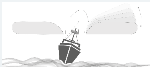
L-IESA non-rotating IFF features beam agility in elevation to compensate ship rolling movements
